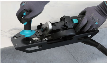
Step 3. Move forward steadily to make a perfect bevelling.
